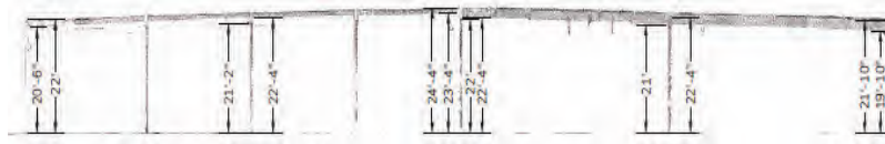
Clear-Heights in Warehouse Area
