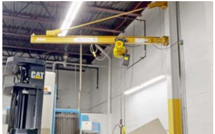
1-Ton Jib Crane - ±10'0" Under Hook (Bay 2)
