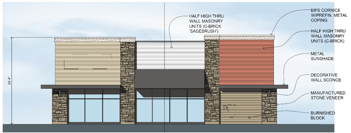
Bldg. A - East Elevation 1/8" = 1'-0"
