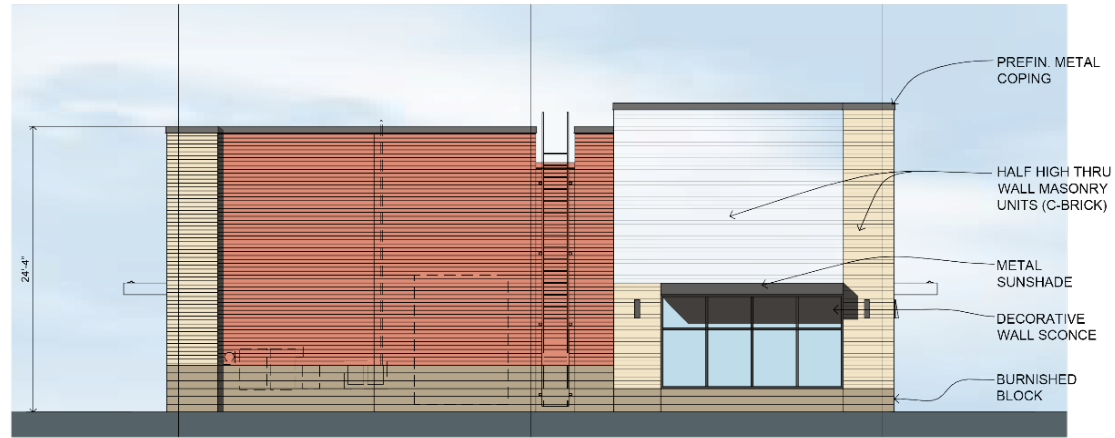
Bldg. A - West Elevation 1/8" = 1'-0"
