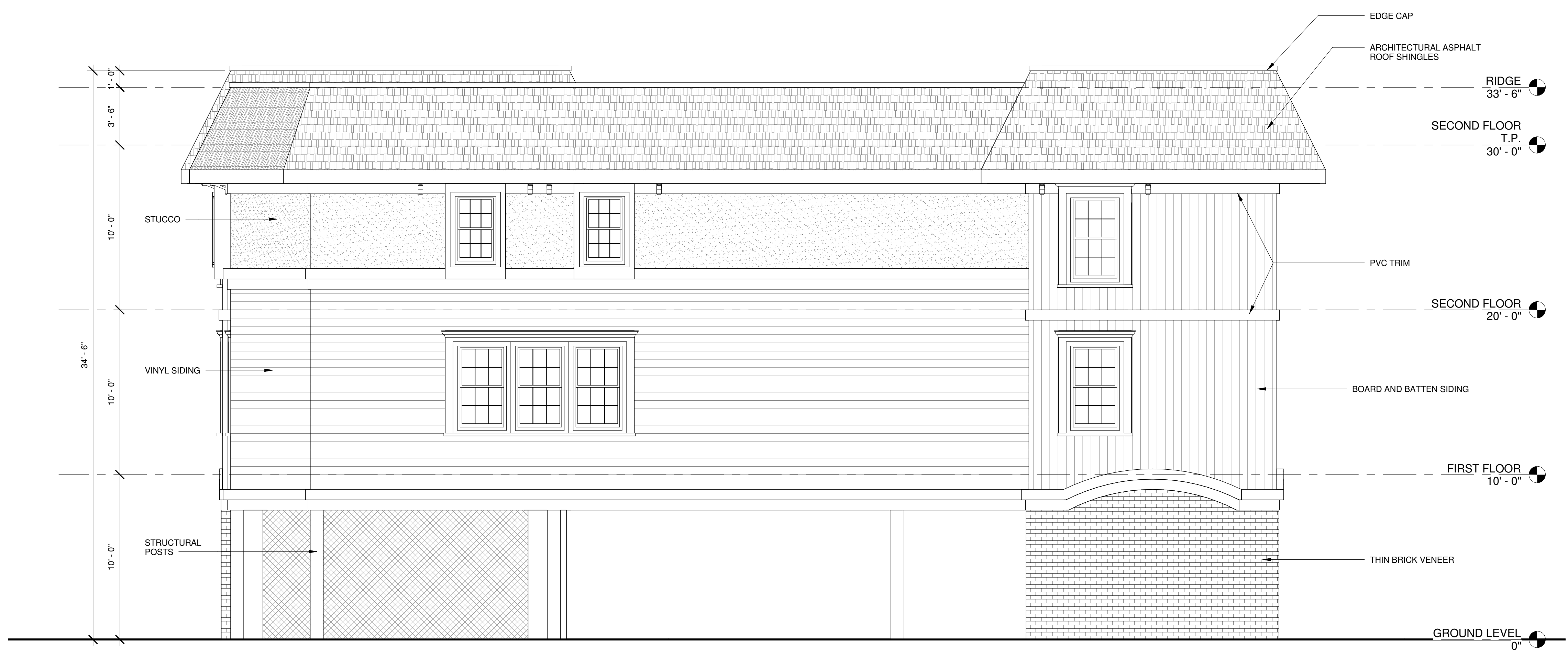
1 SOUTH ELEVATION A-2.2 1/4" = 1'-0"
