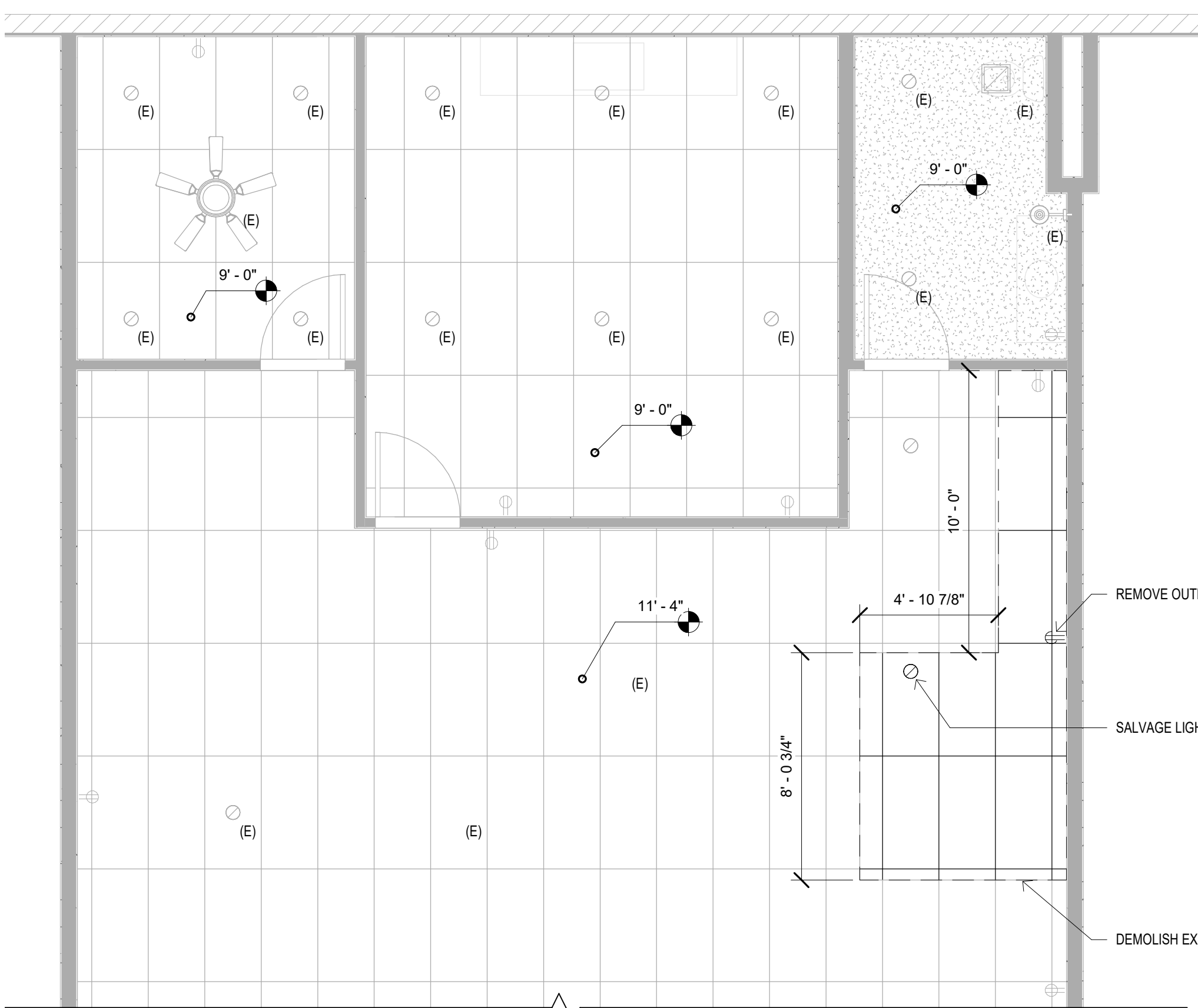
DEMOLITION PLAN SCALE: 1/4" = 1'-0"
